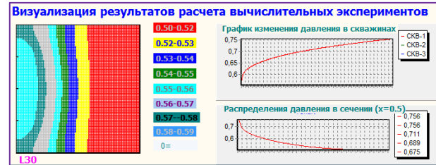
Fig. 2. Change in pressure in an oil reservoir during contour one-sided water flooding
